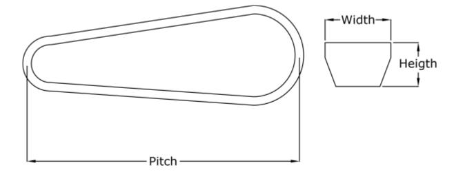
$\begin{array}{ll} \text{Datum Llength} = 4470 \\ \text{Height} &= 10 \\ \text{Length inside} &= 4445 \\ \text{Type} &= \text{BB173} \\ \text{Width} &= 17 \end{array}$
